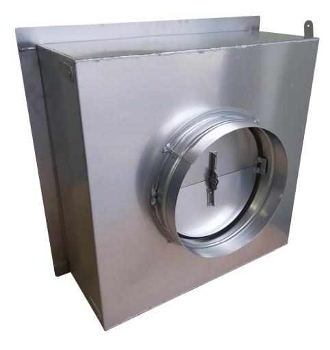
Inlet View (*pic at left*) of **RTM module** showing ribbed duct-collar and the standard damper, a room-side accessible cable-operated butterfly damper. The continuous welded-seam is clearly visible along the top side of the module. The standard module is .063" (16-gage) mill-aluminum, with 304SS as an available option. Also visible are the four corner-mounted hanging tabs and the ribbed collar.
