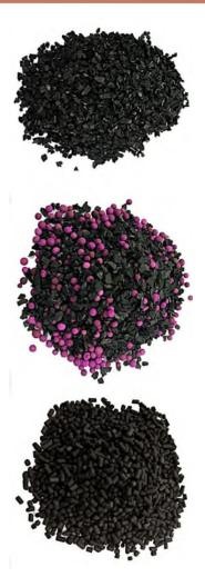
**HEGA (H**igh-**E**fficiency **G**as-Phase **A**ir**) Medias** are various granular and pelletized medias that can put into perforated trays or canisters. Media selected is based on the gaseous-contaminants that are to be addressed. Sometimes medias must be put into consecutive beds to address gaseous-compounds or for high concentrations of certain gases or compounds.
