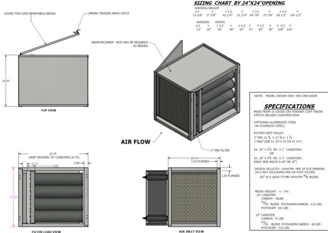
Standard housing is approximately 33" deep (in direction of airflow) when using a 2" deep ASHRAE prefilter and 24" extended-life canisters. Custom filter configurations (multi-pass, etc.) and sizes are available.
