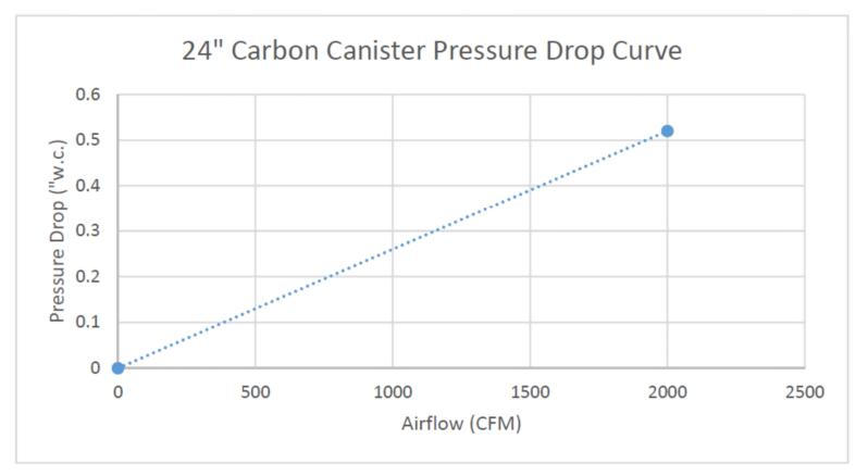
Important Note: Pressure Drop based on quantity (16) canisters in 24"x24" face area
