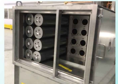
HEGA (Carbon) Canister Odor-Control Unit
