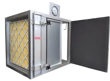
Housings have doors on both sides, and doors have outward-turned flanges and gussets to ensure rigid and durable construction. All filter access doors are fully gasketed with 0.25" thick closed-cell neoprene to ensure leak-free operation at +/-6"wc operation. Door latches are heavy-duty spring-load star-knobs on 0.25" thread.
