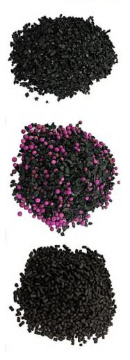
**HEGA (H**igh-**E**fficiency **G**as-Phase **A**ir**) Medias** are various granular and pelletized medias that can put into perforated trays or canisters. Media selected is based on the gaseous-contaminants that are to be addressed. Sometimes medias must be put into consecutive beds to address gaseous-compounds or for high concentrations of certain gases or compounds.
