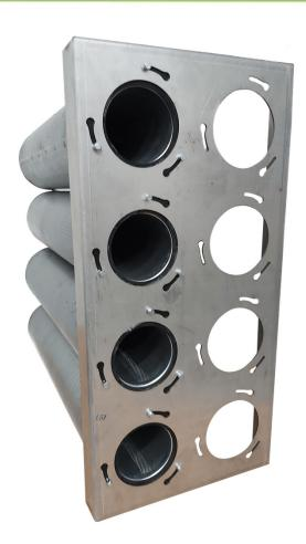
(High-Efficiency Gas-Phase HEGA Air) **Canister Filter Housings** utilize a heavy-duty 12"x24" holding frame to hold the canisters and allow for high-airflow with very low pressure drop. The canisters are gasketed on the side-wall and then slid into the 2" deep filter channel to provide a bypass-free installation in the side-access housing. Canisters are perforated on both the inside and outside and can accept any type of granular or pelletized gas-phase media.
